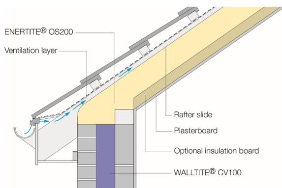
Diagram 2 - Detail of pitched roof with counter battens
